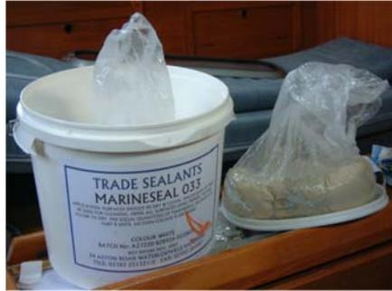
Figure 12: Window 2 Part Putty Sealant
