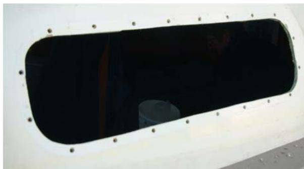
Figure 11: Main Cabin Window: Cut-out, Outside View
