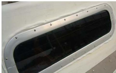
Figure 13: Main Cabin Window Inserted
