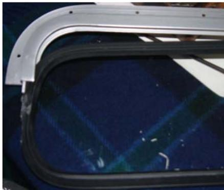
Figure 8: Inserting Glass & Rubber Seal into Frame
